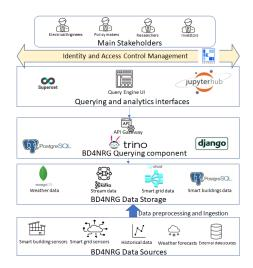
Figure 1. BD4NRG query engine high-level architecture
